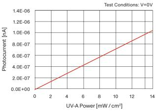
Optical Source: UV-B Lamp (306nm)
