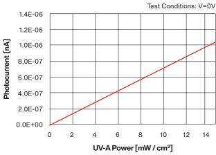
Optical Source: UV-B Lamp (306nm)
