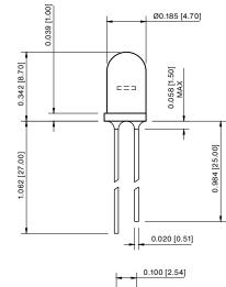
ANODE Note: Lead soldering temperature (5mm from body) 260°C for 5 sec.
