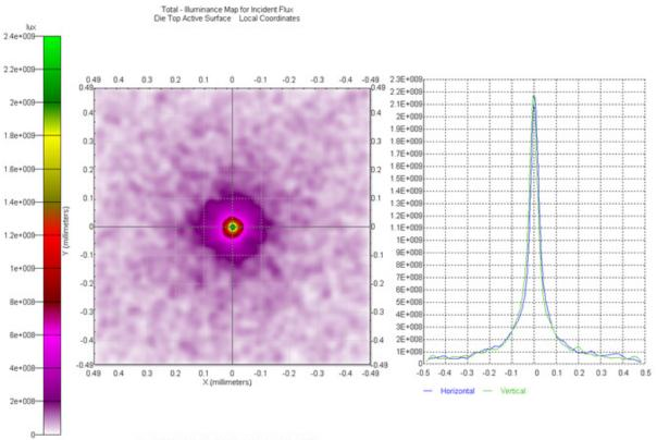
Min:1.0063e+007, Max:2.2519e+009, Ave:8.24e+007 Total Flux:77.531 Im, Flux@mitted Flux:0.11595, 16763 Incident Rays
